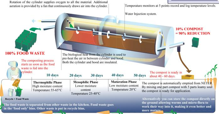
The Neter combines nature and engineering to provide an in composting system that not only converts all food waste to compost also reduces it in weight by up to
